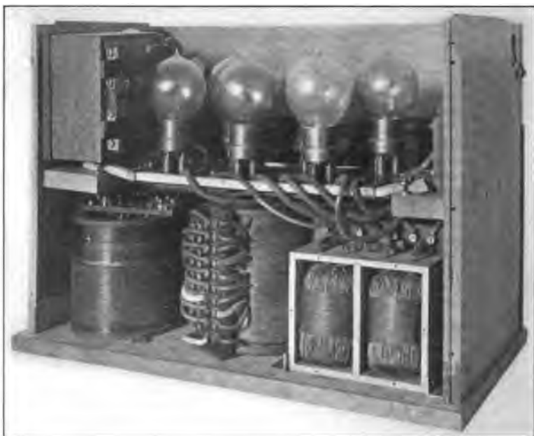
Plate 10. —A typical undamped wave two-way set of French design. Note that the six vacuum tubes used as detector, oscillators and amplifiers are all identical. The amplifier iron core transformers are seen at the lower right hand corner, and at the left are the transmitting and receiving inductances.
